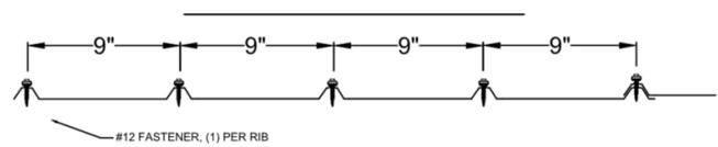
29GA (MIN) ON 18GA (MIN) STEEL FRAMING
