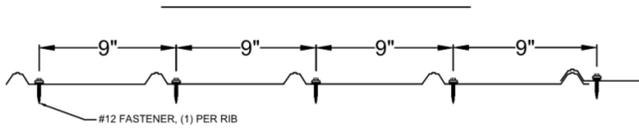
26GA (MIN) ON 16GA (MIN) STEEL FRAMING
